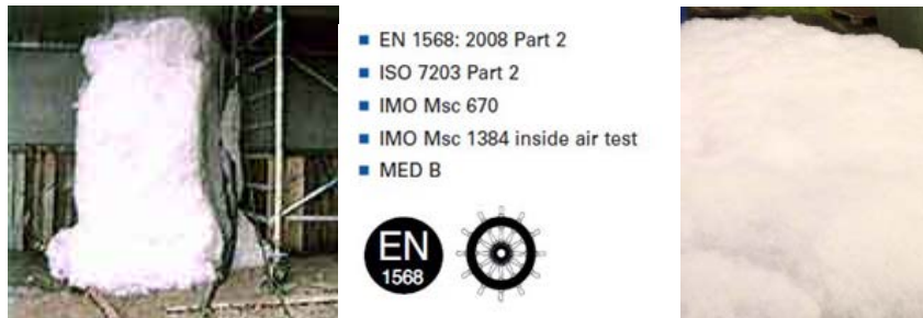
Source: right Li-Ion-Battery covered in Nordhausen –Envites Energy
